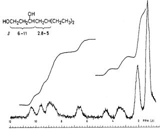
Figure 1.—60-MHz nmr spectrum of deuterated 45 (12 mg) in CCl<sub>4</sub> (150  $\mu$ l) after addition of Eu(dpm)<sub>3</sub> (30 mg).
